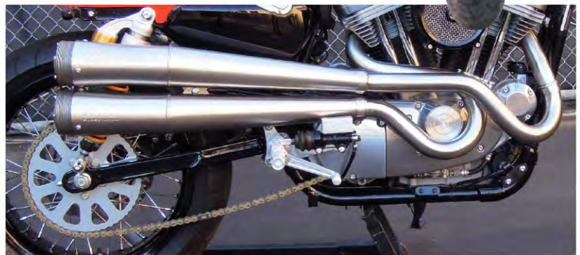
Supertrapp Flat Track Style Exhaust for 2004 to Current Sportsters Note: Intended for use on closed course competition motorcycles only
