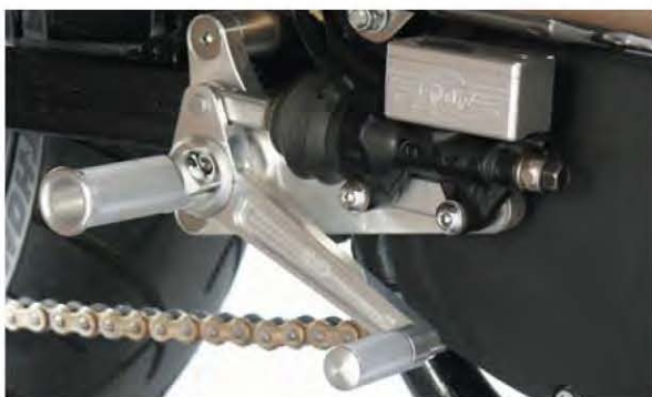
2004-Present left side, std. shift pattern for high or low pipe.
